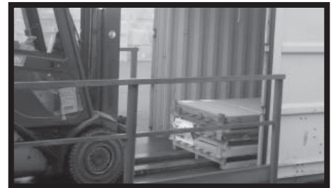
Fig.8 - To take on pallets from their short side (e.g. when unloading containers), use forks with a length of at least 2,5 metres to guarantee a sufficiently long supporting surface and to protect the package and its contents.
