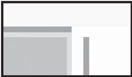
3 - Lay the first slab.
