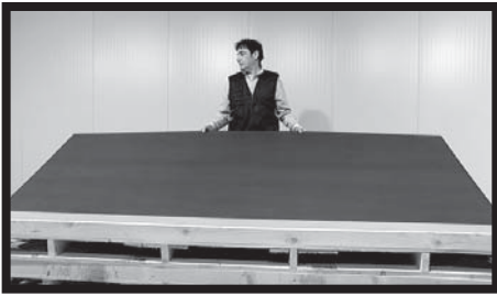
Fig.1 - All types of 300x100 cm KERLITE slabs can be lifted by one person. Lift the slab with open hands. Slowly raise the longer side so as to eliminate the suction effect, due to contact with the underlying slab, and ensure a good grip.
